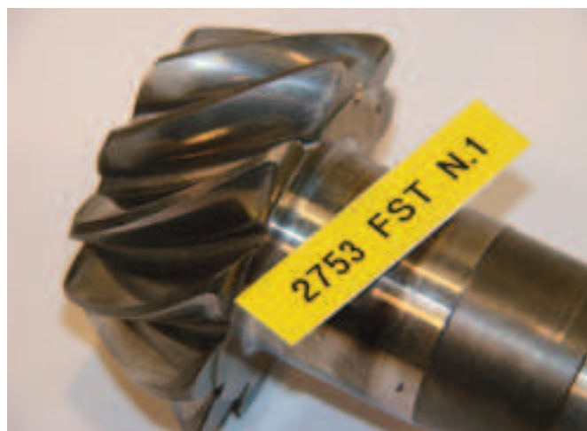
Figure 3 - Teeth wear of the Carraro ORIGINAL pinion at the end of the test
