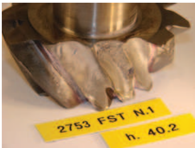
Figure 2 - Teeth base breaking of the NON-ORIGINAL pinion
